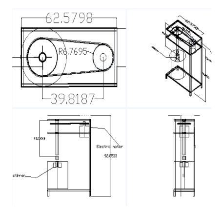
Figure 1: Assembly and isometric drawing of the mixer.
