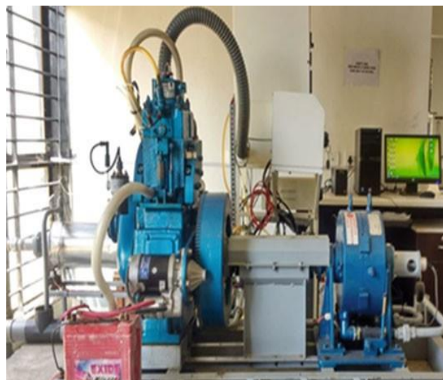
Figure 1: Engine test setup photo (Kirloskar AV-1)
