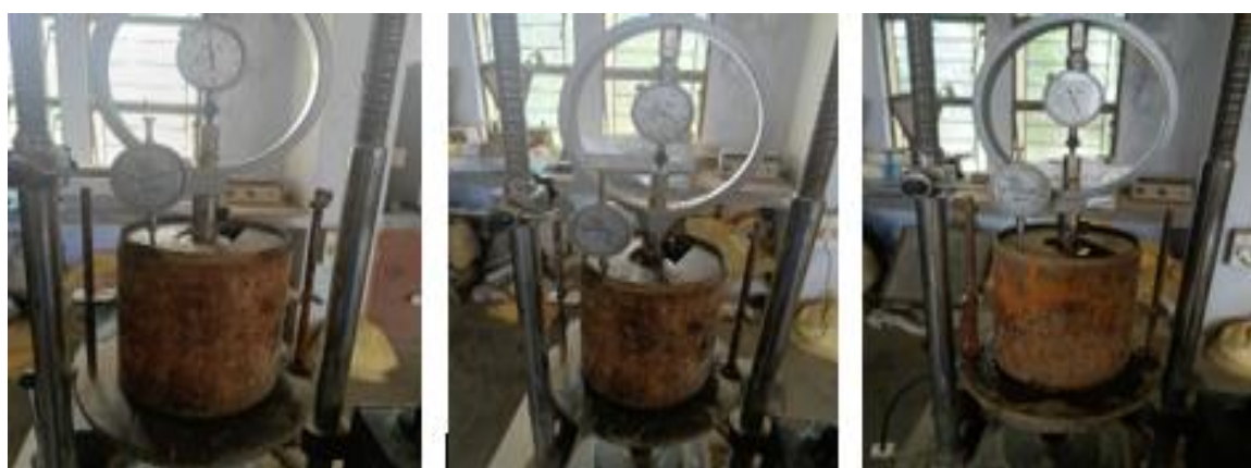
Figure 4: Prepared soaked and unsoaked CBR samples
