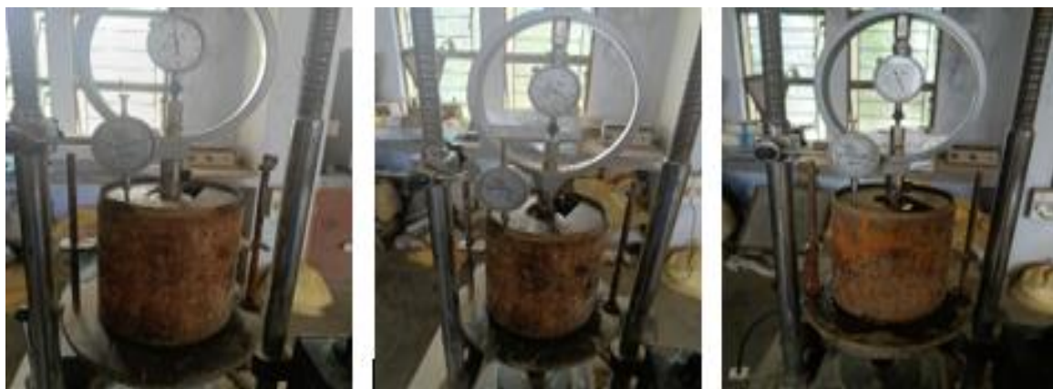
Figure 4: Prepared soaked and unsoaked CBR samples
