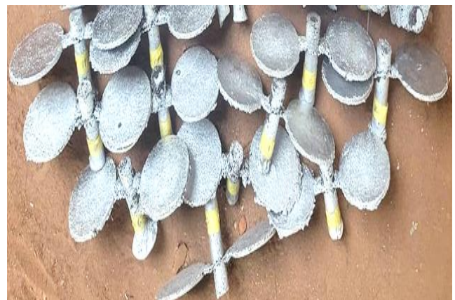
Figure 2: Specimen for wear rate test
