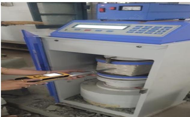
Figure 2(a): R_s test performed on cube specimen
