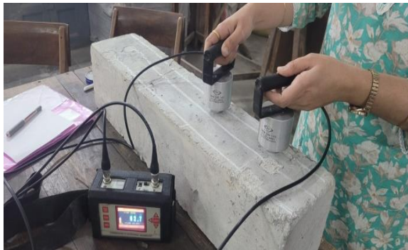
Figure 2(c): V test performed on RC beam at the location of the bar
