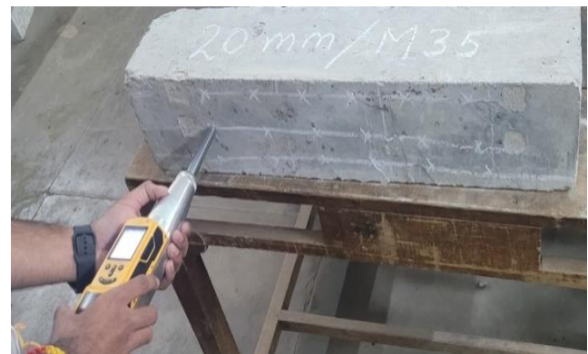
Figure 2(b): R_s test performed at the location of the bar
