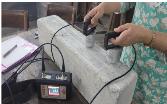
Figure 2(c): V test performed on RC beam at the location of the bar
