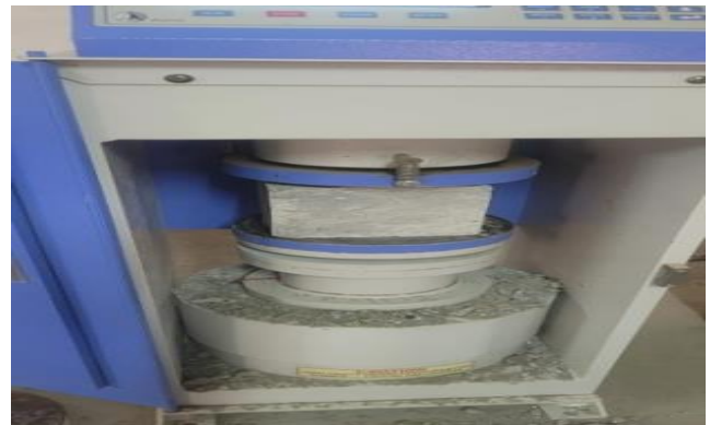
Figure 2(d): Destructive Test on companion Cube
