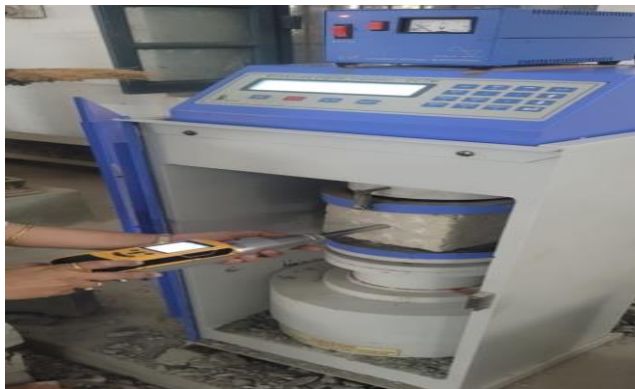
Figure 2(a): Rs test performed on cube specimen
