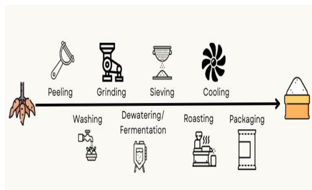
Figure 1: Flow diagram for garri processing [23]
