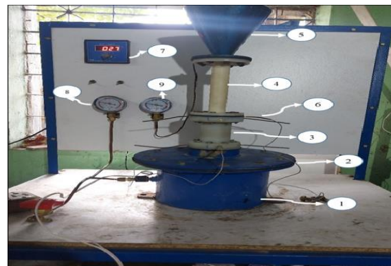
Figure 2: Experimental setup of thermoacoustic refrigerator
