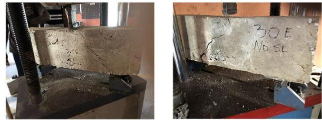
(a): DB7 (30% EPS, 0% TF, No SL) (b): DB8 (30% EPS, 0% TF, SL present)
