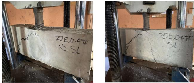
Figure 8: DB5 and DB6 at failure under static loading
