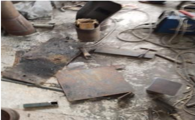
Figure 2: Cutting of the steel plate into small coupon sizes
