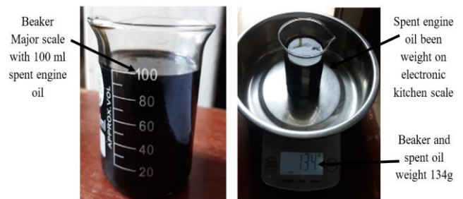
Figure 4: Determining the density of the filtered Spent Engine oil
