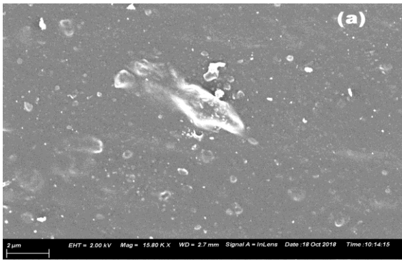
Plate 5: (a) Shows SEM micrograph of composites stirred at 700°C containing 6 wt% SiC and (b) shows the particles distribution using analyser
